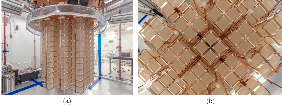
Figure 3.10: Side view (a) and bottom view (b) of all 19 towers of CUORE suspended from the cryostat.
