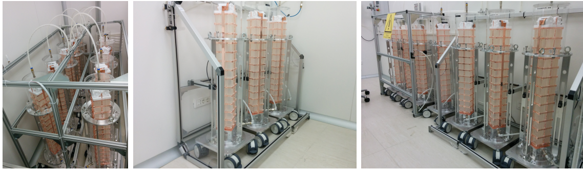
Figure 3.8: Completed CUORE towers were stored in CR4, in special containers constantly flushed with nitrogen, until they were ready to be mounted to the cryostat.
