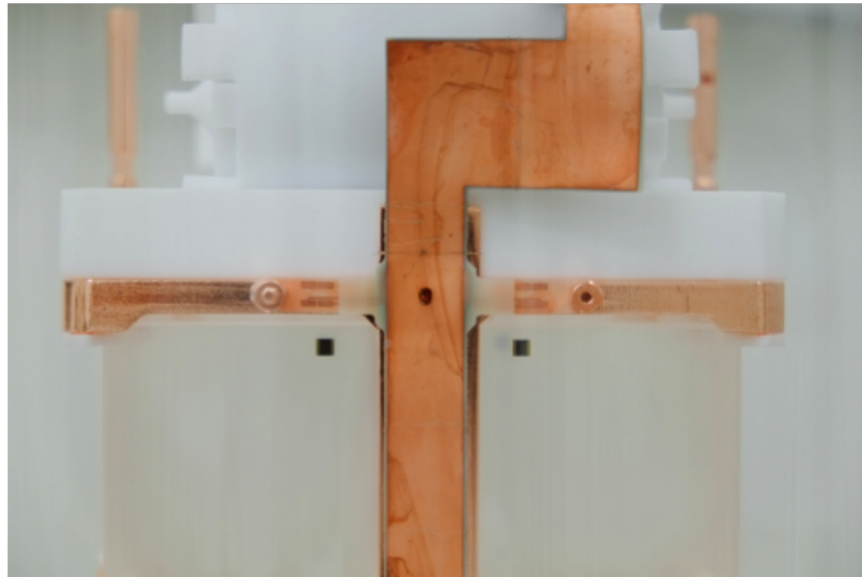
Figure 3.5: Photograph of the top of the CUORE-0 tower, zoomed in to see one of the flexible PCB strips that runs along the length of the tower.
